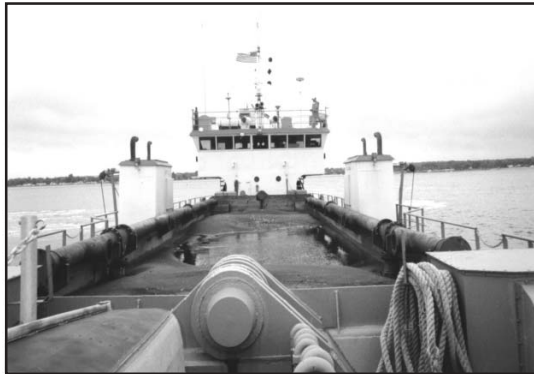
Sand dredged from Clinton Harbor is transported aboard the U.S. Army Corps of Engineers dredge Currituck.
