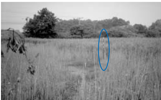
Reference monitoring stake in Hammock River wetlands, Clinton, records the height reduction of common reed over time. The topmost mark shows the height of common reed before restoration. The second, third and fourth marks indicate the height at the end of the growing season in 1985, 1986 and 1987 respectively. Photo (1988) shows the replacement of common reed by salt-marsh cordgrass ( Spartina alterniflora ).
