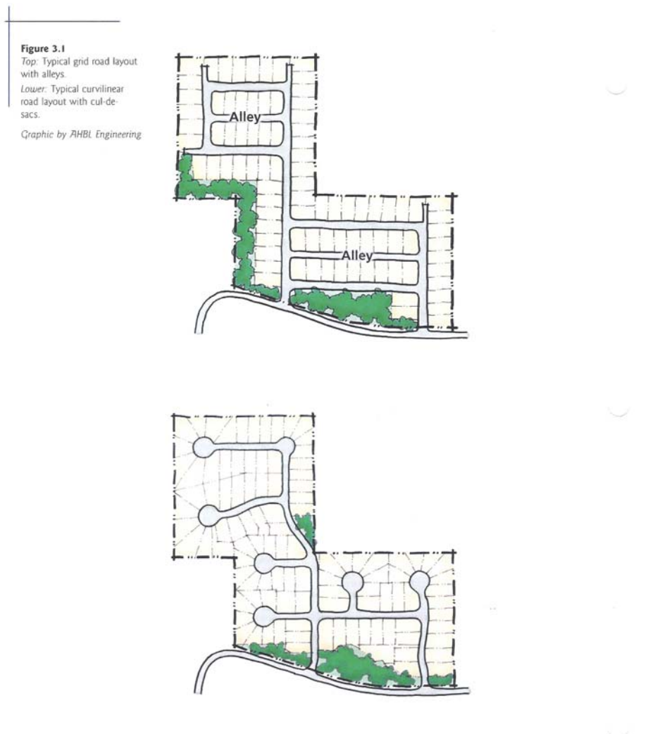
Figure 2 – Typical Grid & Curvilinear Road Alignments
