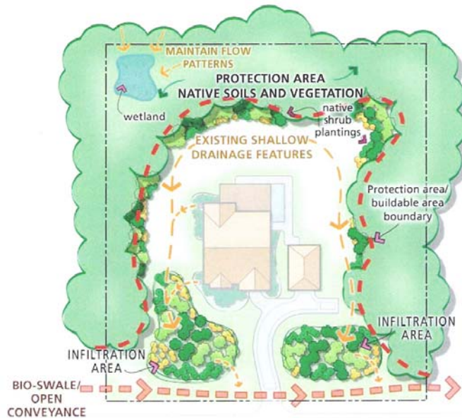
Figure 5 – Sketch showing incorporation of LID storm water measures on a single family lot
