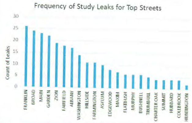
Figure 3. Frequency distribution by street name of Leaks from this study between February 25 through March 31, 2016. A total of 716 gas leaks were recorded in the city of Hartford.
