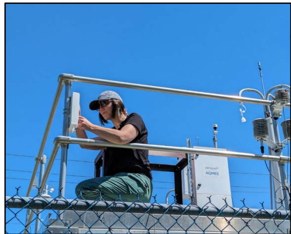
Right: Installation of low-cost air sensor used in collocation studies at East Hartford monitoring site
