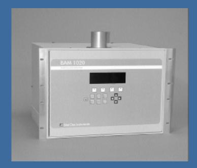
DEEP operates eleven continuous PM monitors at nine sites. This network includes continuous MetOne BAM 1020PM2.5 samplers at each of the nine sites, and paired continuous MetOne 1020 BAM PM10/ PM10-2.5 samplers at the two Ncore sites (New Haven and Cornwall). All BAM monitors are operated year-round and the hourly data is reported to AQS and is used for air quality index (AQI) reporting
