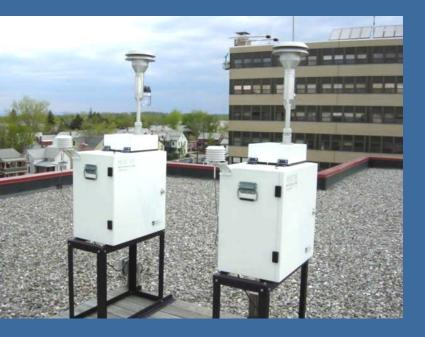
DEEP operates 9 PM2.5 FRM (filter based) sites in the air monitoring network using Thermo Partisol<sup>®</sup>-Plus 2025/2025i sequential air samplers. Two of the sites, Criscuolo Park in New Haven and McAuliffe Park in East Hartford, operate on a daily sample schedule while all the other sites operate on a 1-in-3 day sample schedule.
