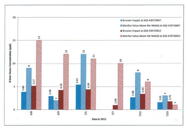
**Figure 8.** Modeled 8-hr ozone impacts from Brunner Island exceeding 1% of the ozone NAAQS, and incremental monitored ozone concentrations above the ozone NAAQS on days when the NAAQS was exceeded at air quality monitors near Lancaster.
