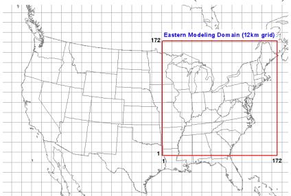
Figure 2-2. Modeling domain used for CMAQ and CALGRID modeling studies. Gridlines are shown at 180 km intervals (15 x 15 12km cells).
