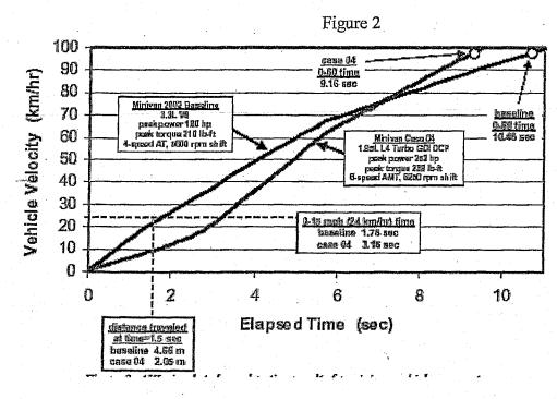
Figure 2: AVL simulated acceleration results for minivan vehicle segment, showing baseline and case 4 (the downsized turbocharged case)
