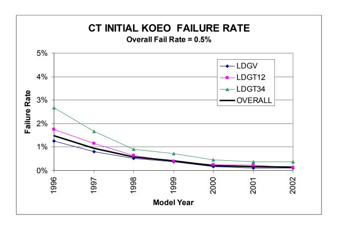
This chart shows failure rates by model year for the Key-On Engine Off (KOEO) test, which is part of the OBD test. The average KOEO failure rate for all vehicles was 0.5%. The Key-On Engine-Off (KOEO) determines if the MIL bulb is working. The bulb should illuminate when the vehicle is turned on but not started.
