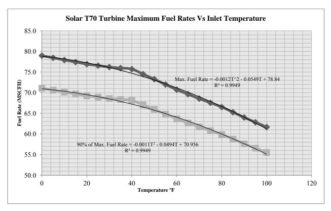
Correlation factor for both equations are closer to 1.0, representing a very reliable prediction of fuel rate based on the ambient temperature. The equations are added to the permit and the charts (as Appendices) can be referenced for more details.
