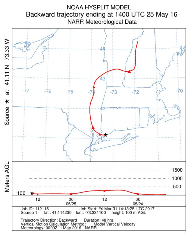
Figure 72. 100 meter Back Trajectory from Westport Connecticut ending at 10:00 am LDT May 25, 2016.
