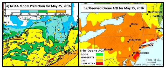
**Figure 1. Model Forecasted Air Quality versus Observed.** NOAA model forecasted AQI values for May 25th, 2016 (a) and the observed ozone AQI values (b). Figure 1a shows the early morning forecast (isopleths) for the day of May 25<sup>th</sup> including wind fields and actual observed ozone AQI levels at monitoring sites (circles) in the northeast. Figure 1b shows the extent of the observed ozone levels. Note that Figure 1a color scheme for monitors match the color scheme in figure 1b.
