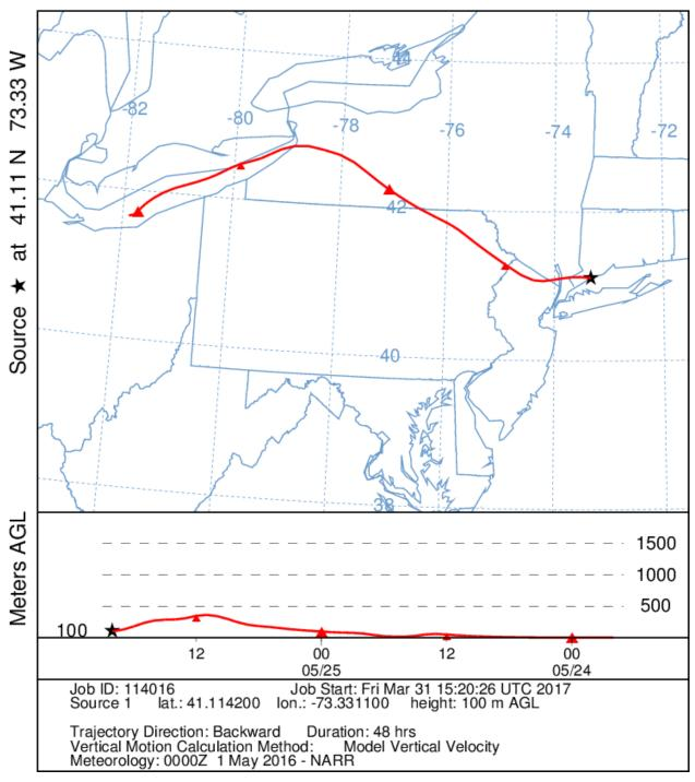
Figure 74. 100 meter Back Trajectory from Westport Connecticut ending at 4:00pm LDT, May 25, 2016.
