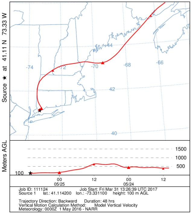
Figure 72. 100 meter Back Trajectory from Westport Connecticut ending at 6:00 am LDT May 25, 2016.
