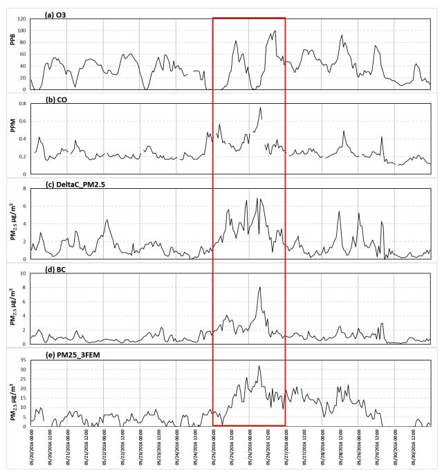
Figure 12. Monitored (a) Ozone, (b) Carbon Monoxide (CO) (c) DeltaC PM2.5 (d) Black Carbon (BC), and (e) PM2.5 at the New Haven CT Monitor
