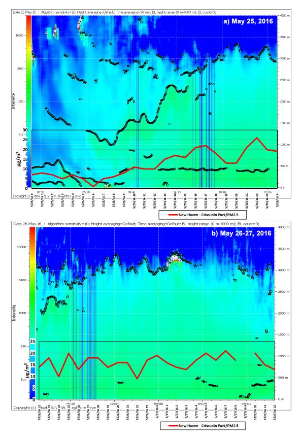
Figure 9. Aerosol Backscatter Intensity over New Haven with PM2.5 Levels
