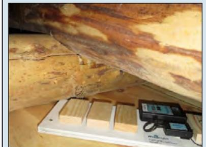
*A climate monitoring panel installed in a historic Norwegian building. Credit: Haugen et al. 2018.*
