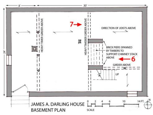
Figure 5a. Basement floor plan, James Alexis Darling House, 1932 Litchfield Turnpike, Woodbridge, CT with photograph key.
