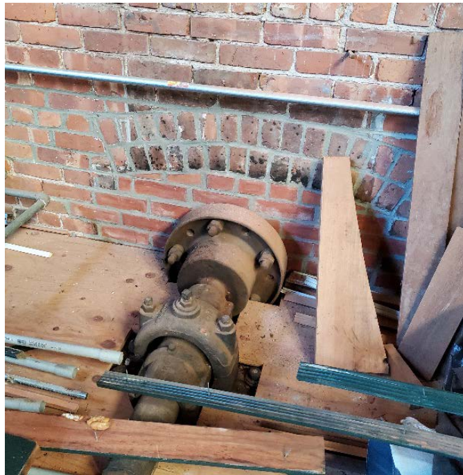
Photographs 55 & 56. Inside the engine block: partial view of turbine pit and outflow flume toward street (L), and power shaft coming off turbine (R).
