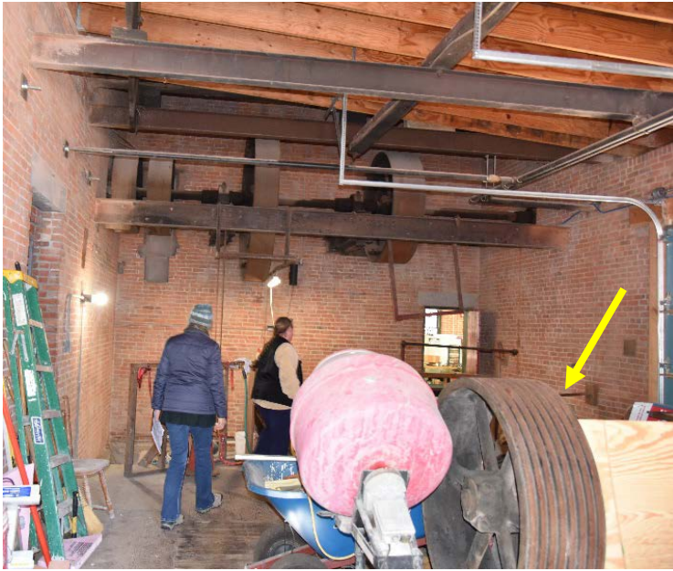
Photographs 57 & 58. Belt shaft and pulley system above turbine pit against far (east) wall in engine block, with additional equipment visible in foreground (L); belt shaft emerging from north wall of engine block into polish room (R).
