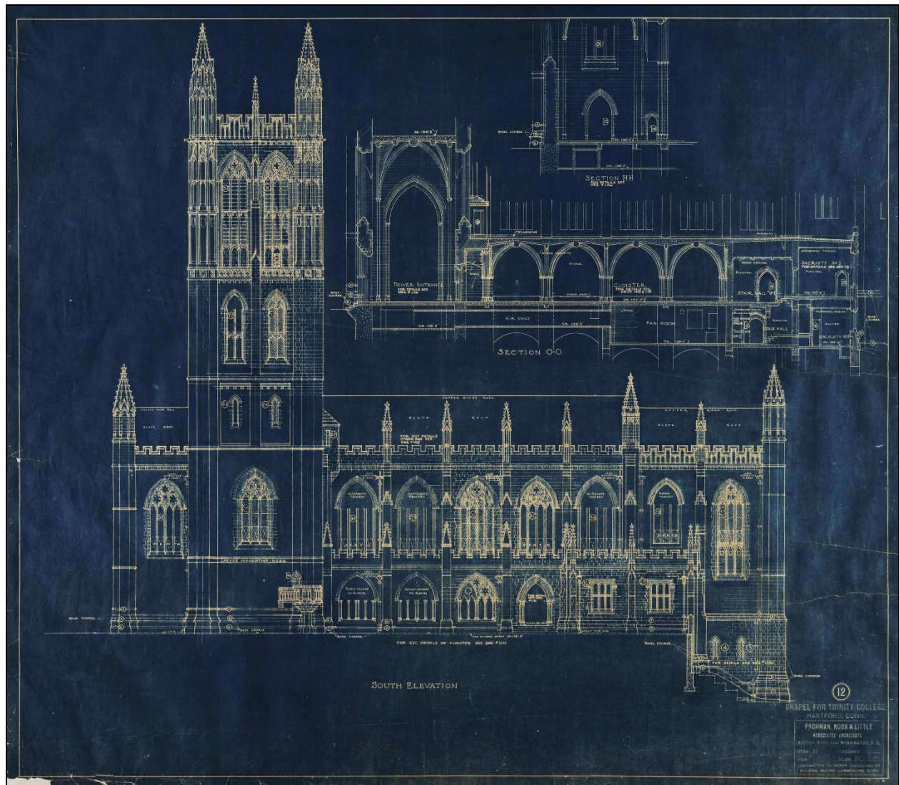
Figure 3. Blueprint of Chapel south elevation and sections, by Frohman, Robb & Little (from Trinity College Watkinson Library and College Archives).
