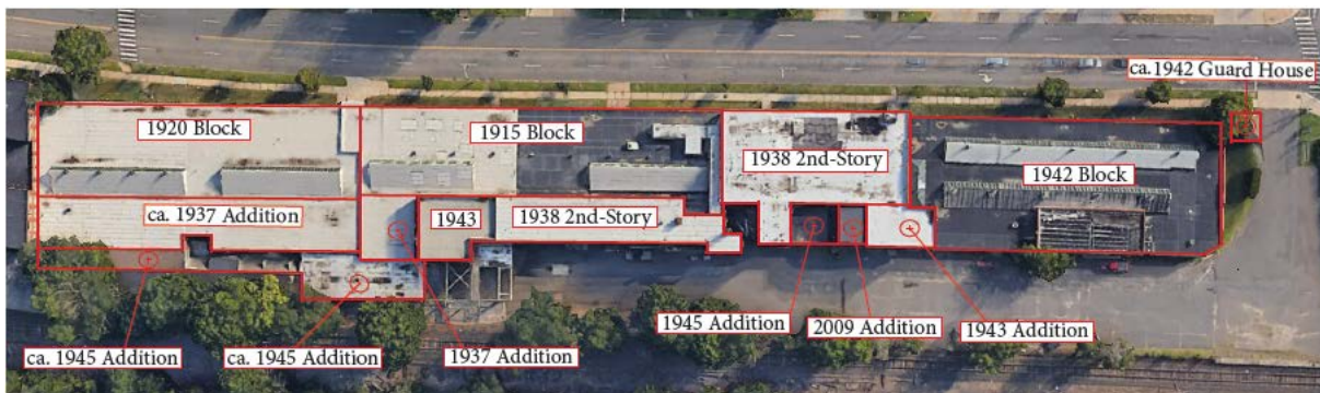
Figure 3: Phases of construction of the Hartford Special Machinery Company.
