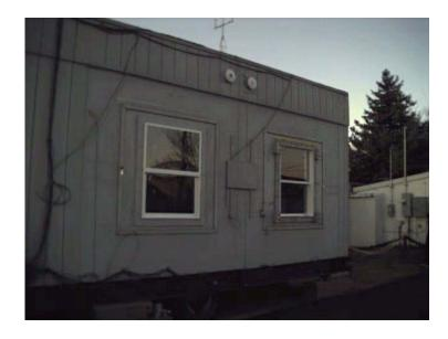
Figure 1. A View of the Test Facility. The faces of the two calorimeter chambers holding the test samples is shown. Left: Chamber B, holding the replacement window; Right: Chamber A with the prime/exterior storm combination. Also are the pyranometer visible pyrgeometer (circular objects at top of wall, center) that measure the incident solar flux and sky temperature, and a portion of the weather tower (top, center) holding the wind speed and direction sensors.
