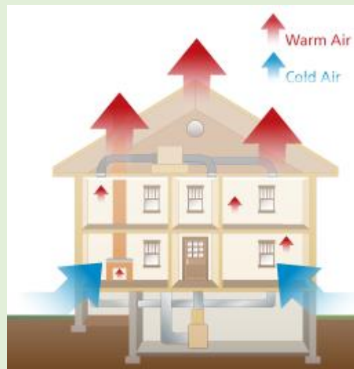
Stack Effect. Source: Blank Space, LLC.
