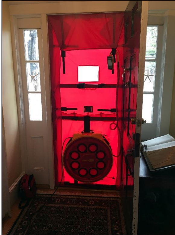
Blower door test. Photo: Marguerite Carnell.
