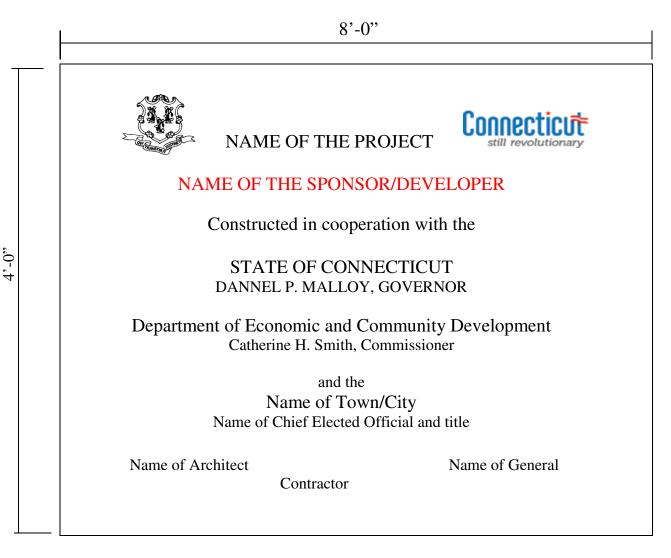
SIGN PANEL: ¾" MDO-EXT-APA PLYWOOD SUPPORTED WITH (2) 4X4 TREATED WOOD COLUMNS AND SECURED 4' INTO GRADE. TOP OF SIGN AT 8'-0" ABOVE GRADE.
