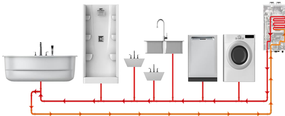
Navien comfort flow illustration Demand recirculation system
