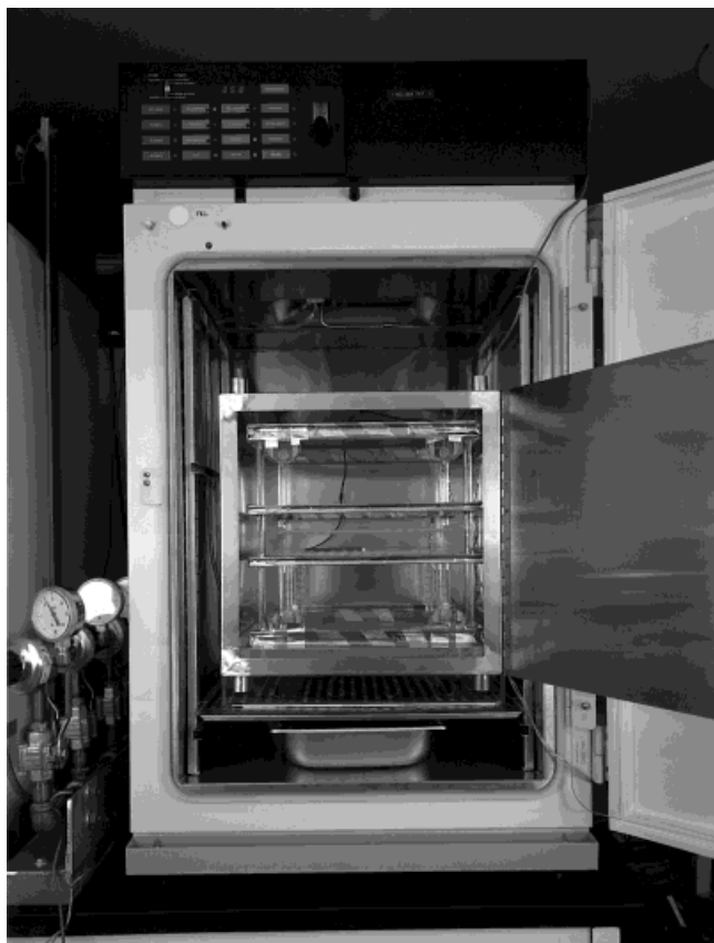
Fig. 1. Cell culture exposure system showing the combination of the 4-square Merritt coil and the mu-metal chamber, which are both placed inside of a commercial cell culture incubator. Also shown is a thermistor temperature probe which is threaded through one ventilation hole into the mu-metal chamber and placed inside the chamber at the position where cell culture plates are typically located. The 4-square Merritt coil can be rotated 90° to reorient the magnetic field vector from the standard vertical position to horizontal.
