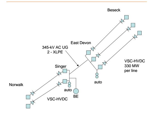
Figure 1. Dual DC Option Configuration
