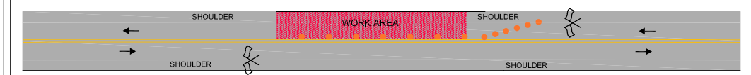
WORK IN TRAVEL LANE AND SHOULDER - TWO LANE HIGHWAY ALTERNATING ONE-WAY TRAFFIC OPERATIONS MAINTENANCE TRAFFIC CONTROL PLAN 13
