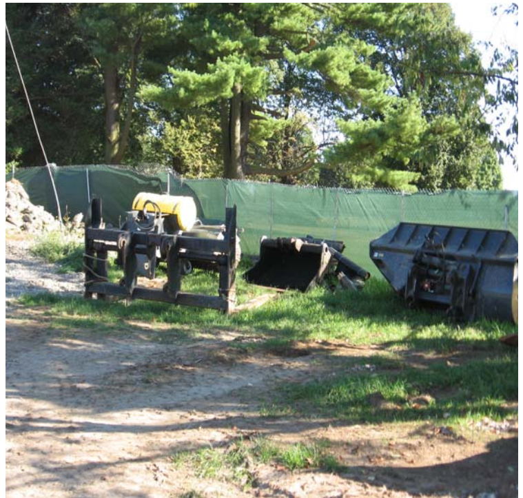
Both photographs were taken within the Sherwood Island lay-down yard. Left: Down limb located near the rear of the yard was removed from the erosion controls. Erosion controls continue to function properly. Right: Fluid filled equipment was being stored on exposed soil in an uncontained/unprotected location.
