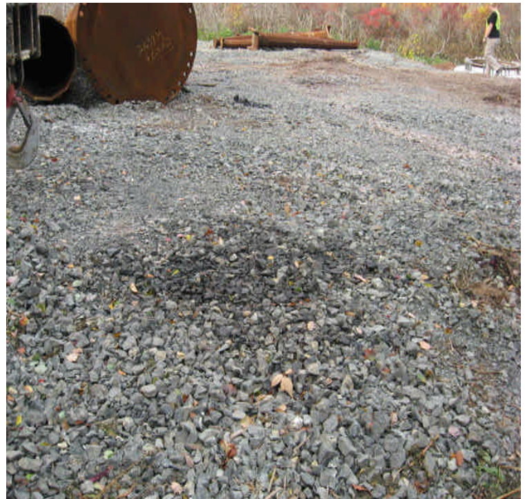
Tamarack Swamp Rd.: One of three stains/drip spots associated with leaking equipment and noted adjacent to the wetlands.
