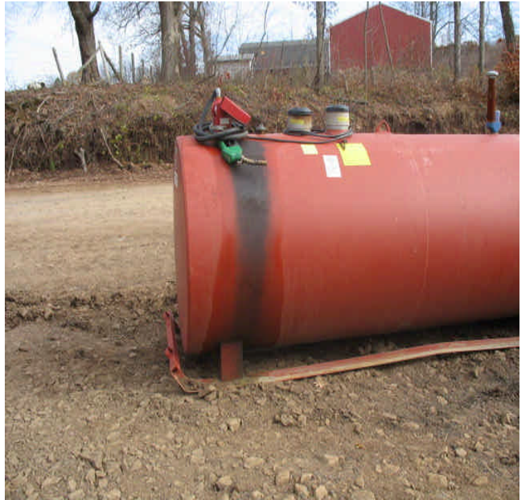
Another fuel tank was being stored at the contractor yard. It was dripping gas along the side with the nozzle facing downward. Consider placing tanks on a liner or similar containment.
