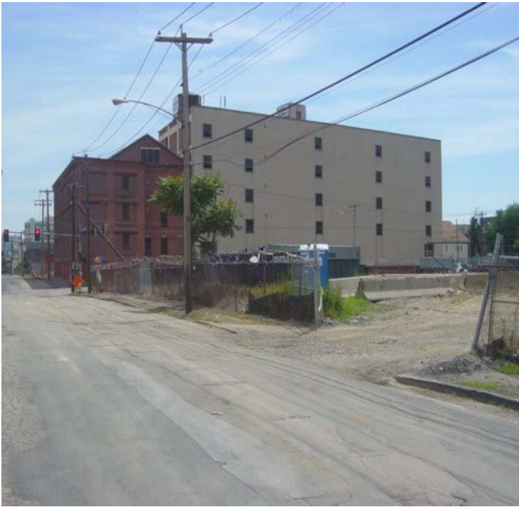
Sediment tracking continues from a storage yard not associated with this project near the intersection of Railroad Ave. and Myrtle Ave.
