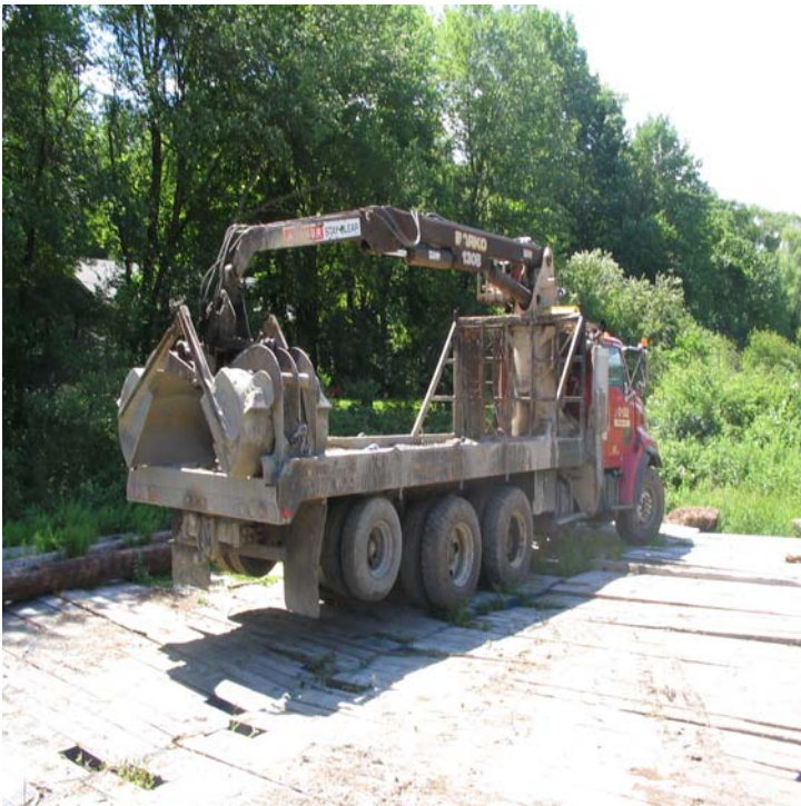
Manville Rd (Woodbridge): Equipment should be parked 100 feet from wetland areas when feasible.
