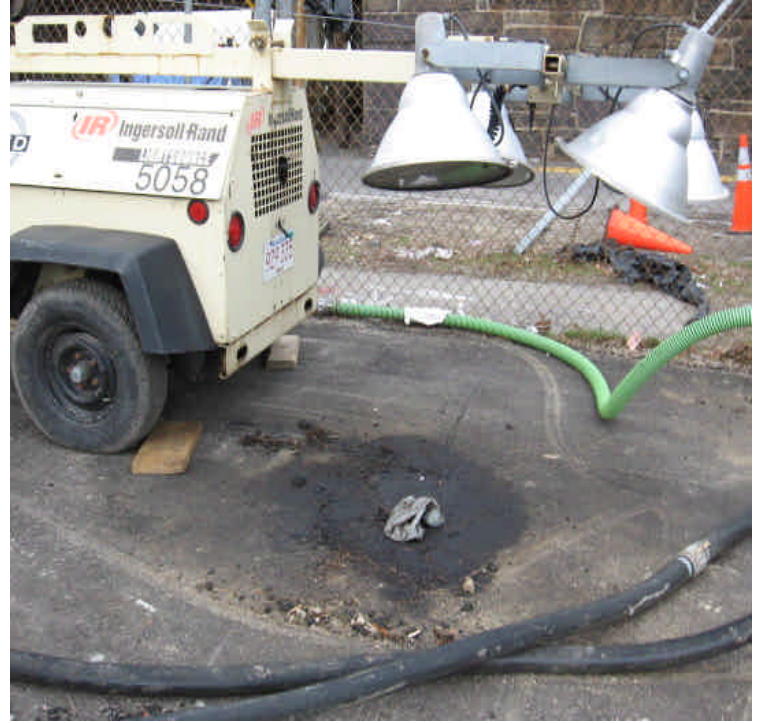
Left: Photo of trenching activities along Railroad Ave. at its intersection with Howard Ave. The sediment on the pavement adjacent to the filter equipment should be swept up and disposed of. Right: Oil spill on the pavement noted next to generator that should be cleaned as feasible.
