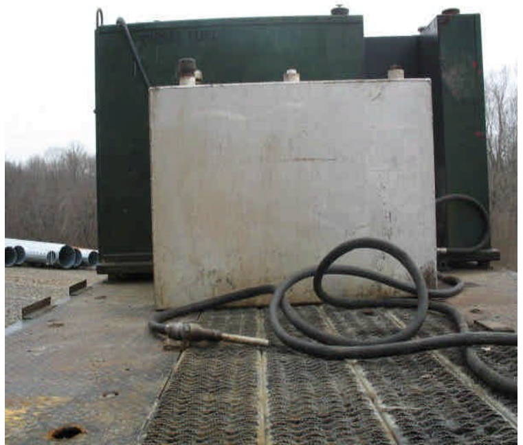
Truck with a portable refueling tank. Nozzle should be contained to prevent spilling. Ensure that spill kits are present on the vehicles.
