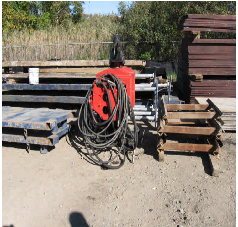
Fluid-filled equipment/attachments located in the yard. The equipment is leaking and is not contained.
