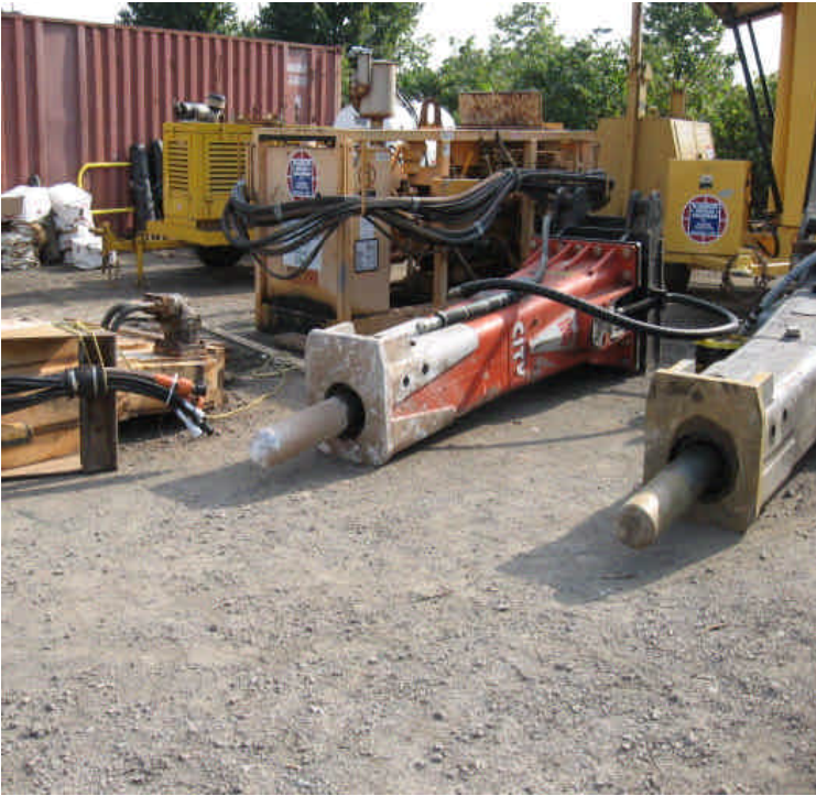
Attachments with fluid-filled hoses are being stored in the yard. In an effort to contain potential spills, equipment could be stored on pads or similar in case of leaks or breakages.
