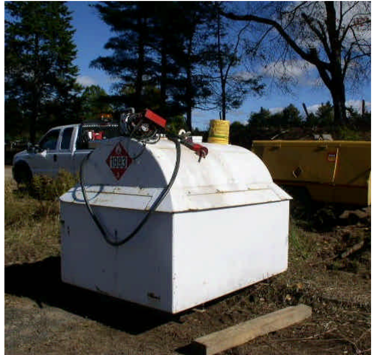
Fuel was observed dripping from the nozzle of a refueling tank at the contractor yard. Controls/improved storage are needed as soon as possible.
