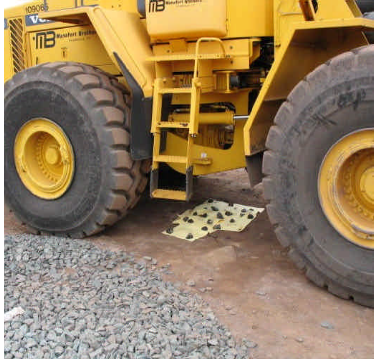
Spill controls being used under a leaking vehicle.
