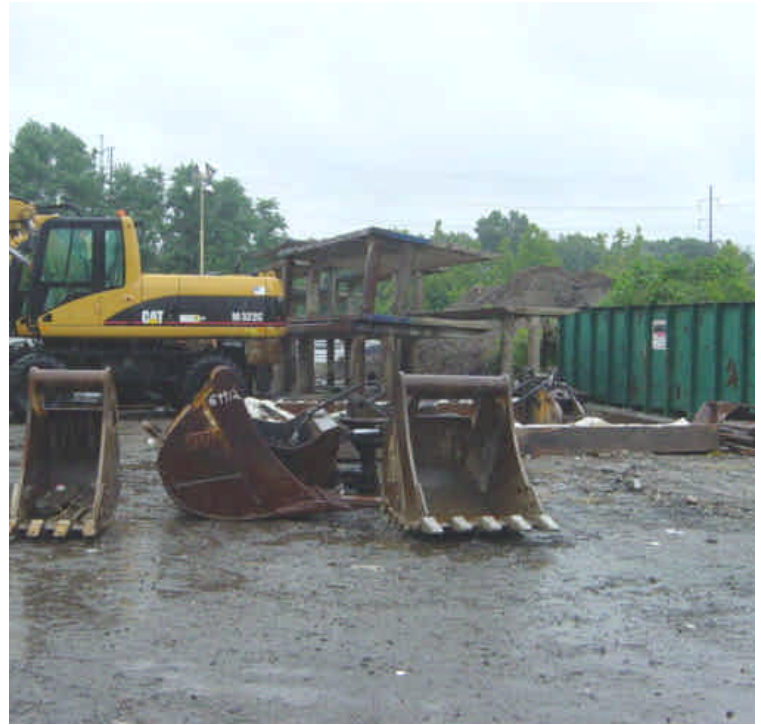
Both photos were taken within the King's Highway lay-down yard. Left: Materials were still observed overwhelming perimeter barrier controls in two locations to the left and right of photo view. Right: A fluid filled bucket/attachment was being stored just outside of the containment area but still within the yard. Continue to store fluid filled equipment proactively within the containment area.
