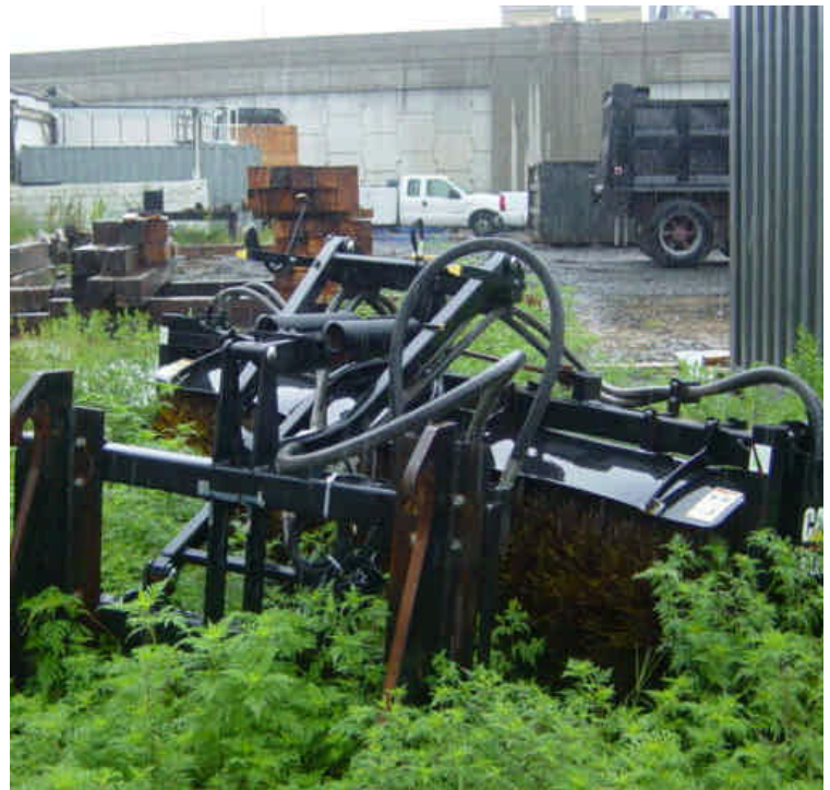
A fluid-filled sweeper was noted stored within the Bostwick Ave. lay-down yard. Continue to store all fluid filled equipment proactively in the proper containment.
