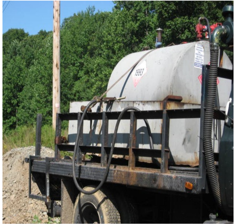
Shunpike Rd: Refueling tank with unsecured nozzle dripping.
