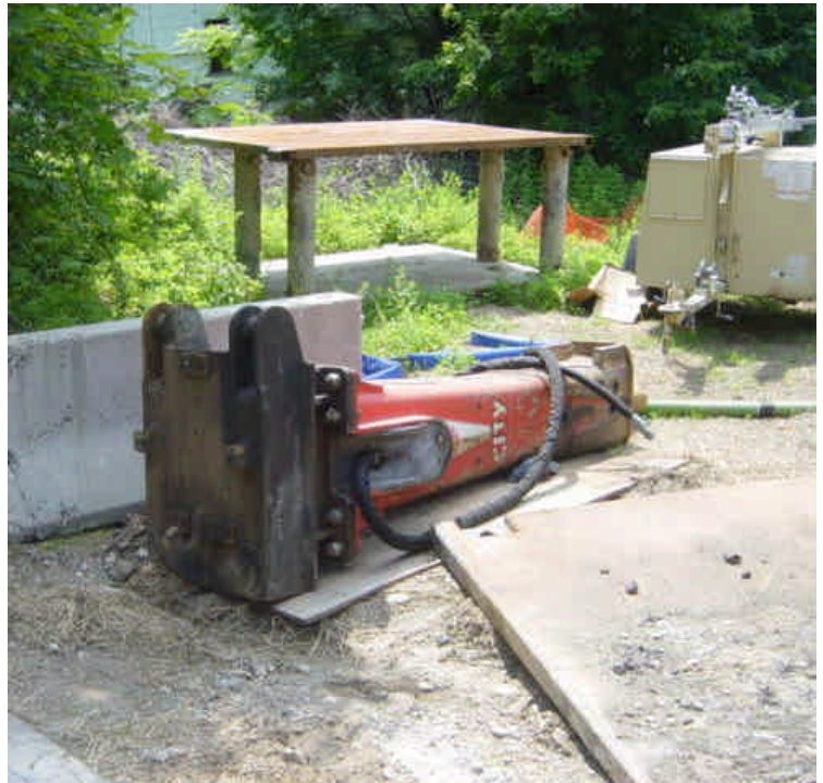
A piece of plywood has been placed under the hydraulic jacking hammer stored near sta. #1020 to proactively contain any potential leaks.
