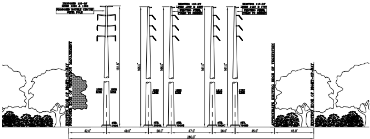
PROPOSED R.O.W. CONFIGURATION DOUBLE CIRCUIT STEEL MONOPOLE DESIGN LOOKING FROM MONTVILLE SUBSTATION TO NORTH OF KITEMAUG ROAD IN THE TOWN OF MONTVILLE, CT STR. #7608
