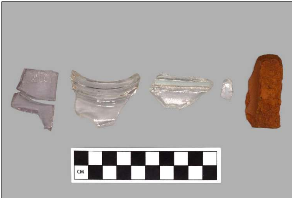
Photo 12. Left to right; two solarized contact molded bottle shards, a machine made jar shard, a pressed, embossed container shard, a contact molded bottle shard, an extruded brick fragment.
