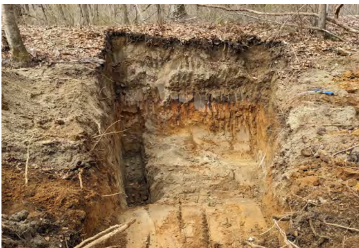
Photo 1: TP-1 bottom and side wall to 10 ft
