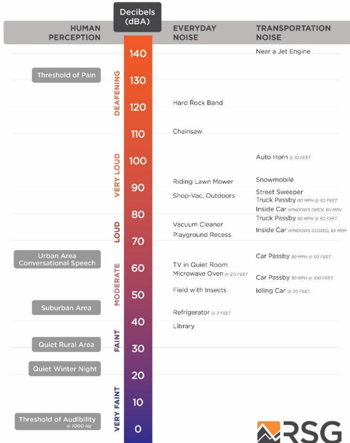
FIGURE 5: A SCALE OF SOUND PRESSURE LEVELS FOR TYPICAL SOUND SOURCES
