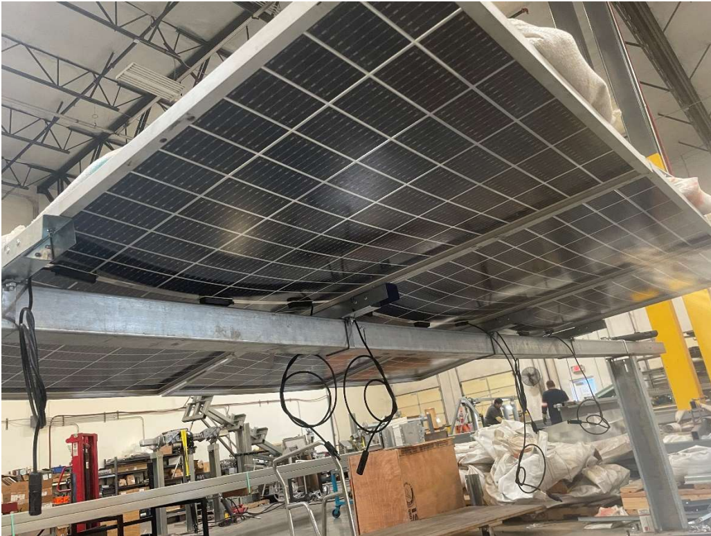
Figure 5: Test table assembly under load
