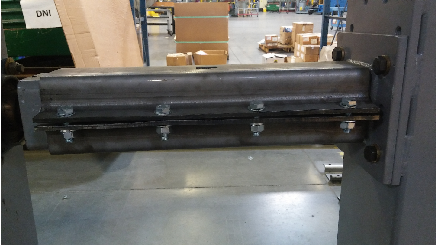
Figure 3: Close-up of Normal Splice Test Sample
