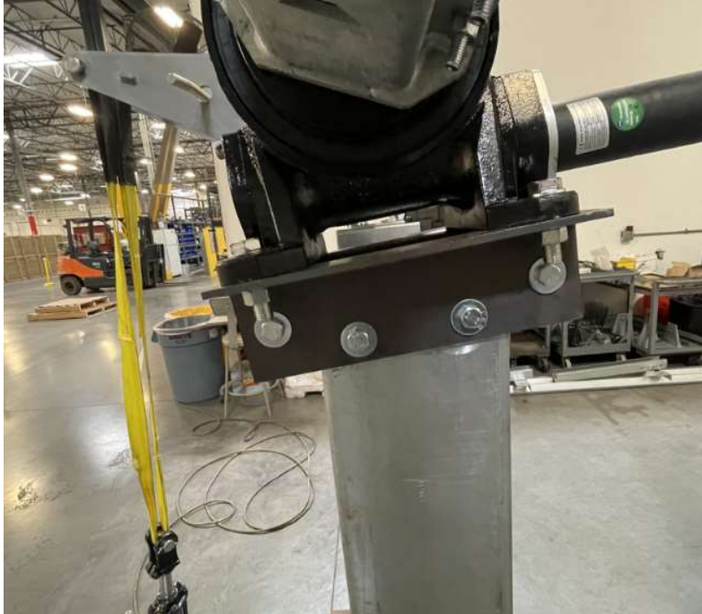
Figure 3: Connection slip at 7,500 ft-lbs w/ standard hardware configuration
