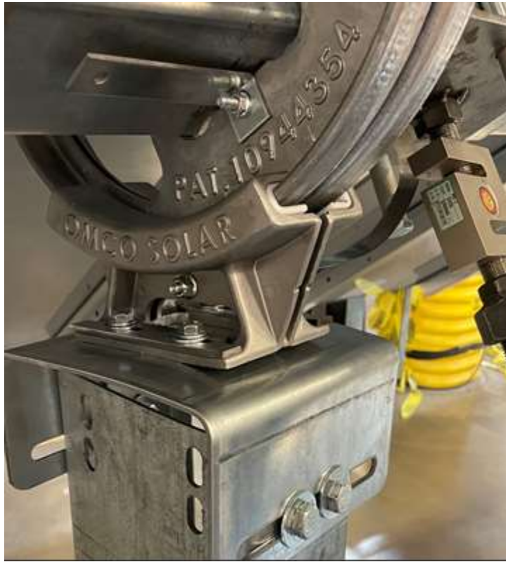
Figure 3: During Max Uplift Loading
