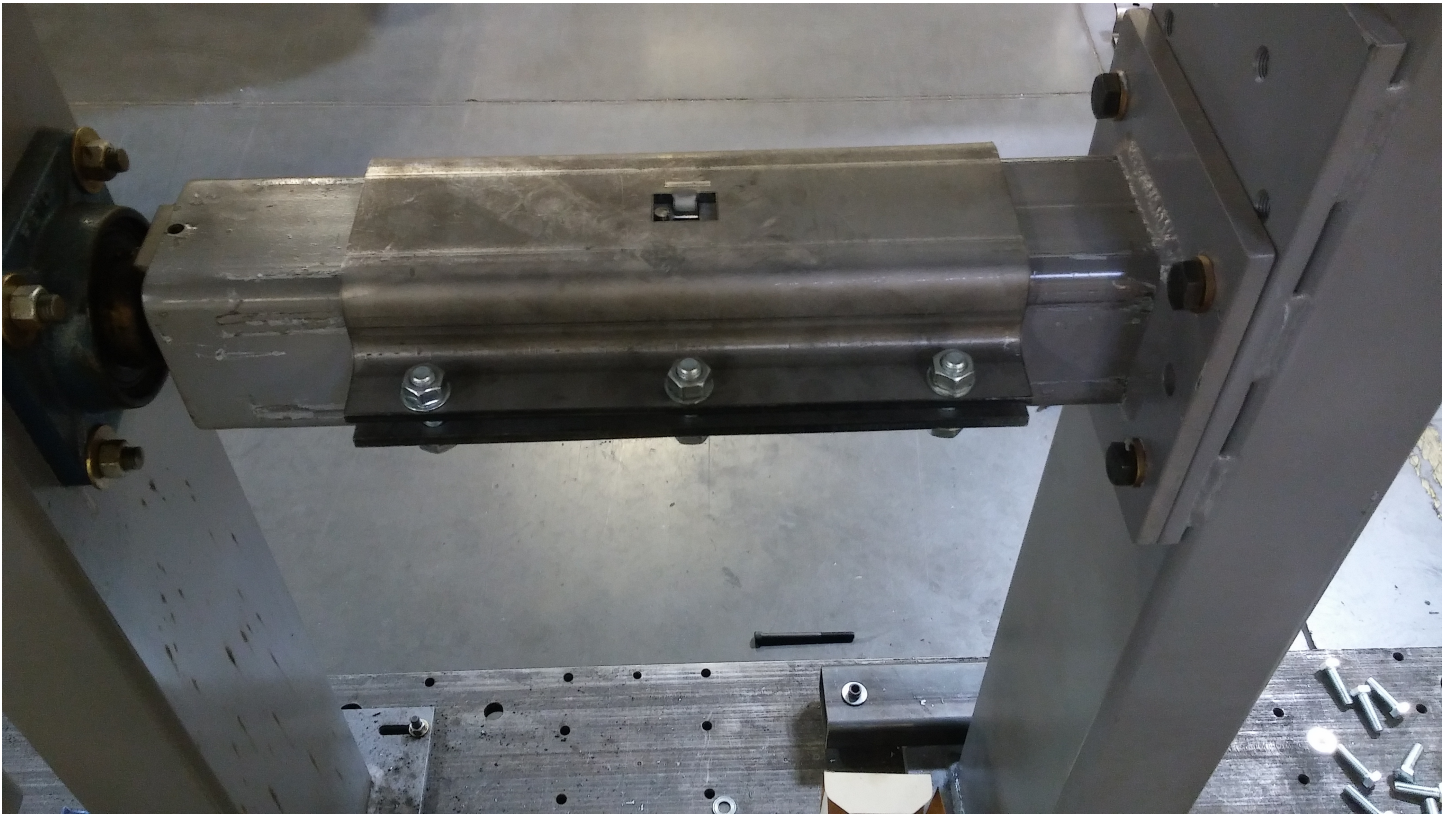
Figure 4: Close-up of Mini Splice Test Sample
