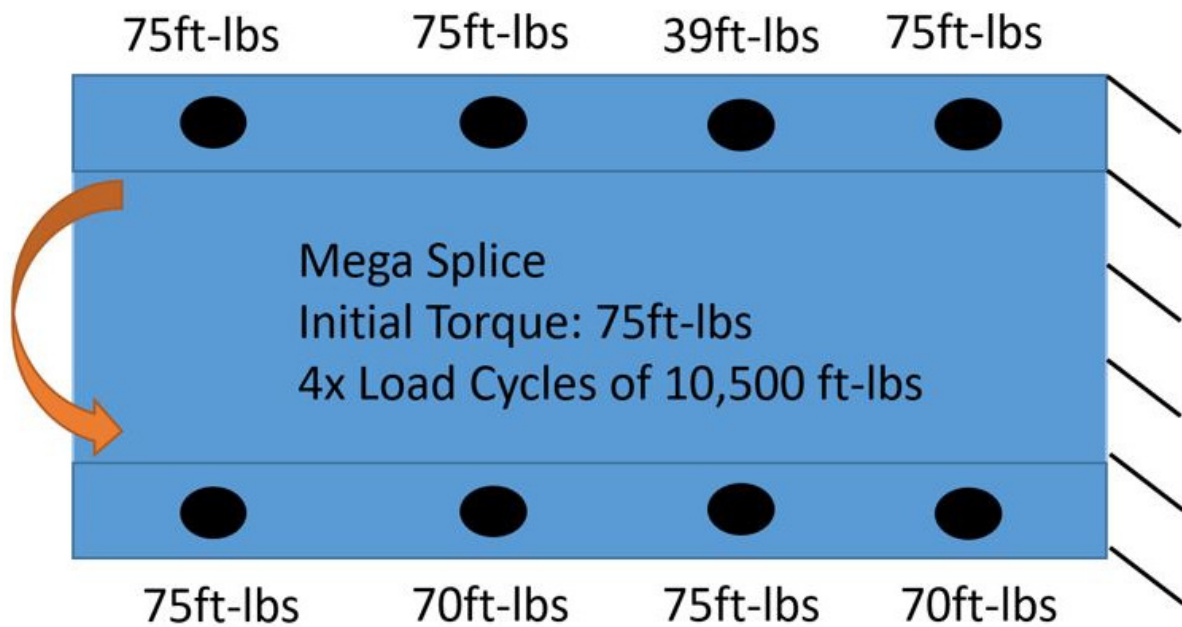
Figure 5: Mega Splice Post-Test Bolt Torque
