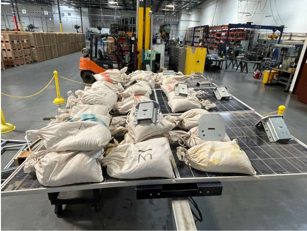
Figure 4: Test table assembly under load
