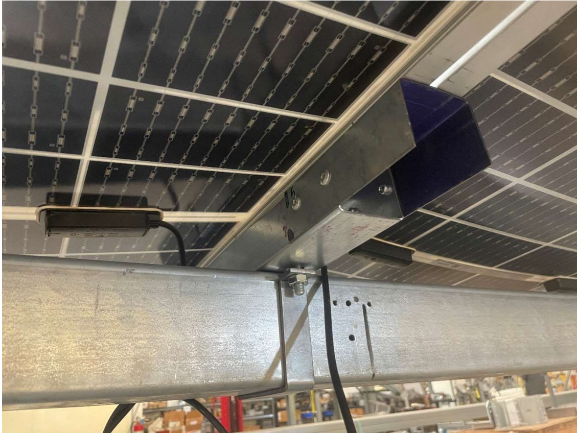
Figure 6: Test table assembly under load
