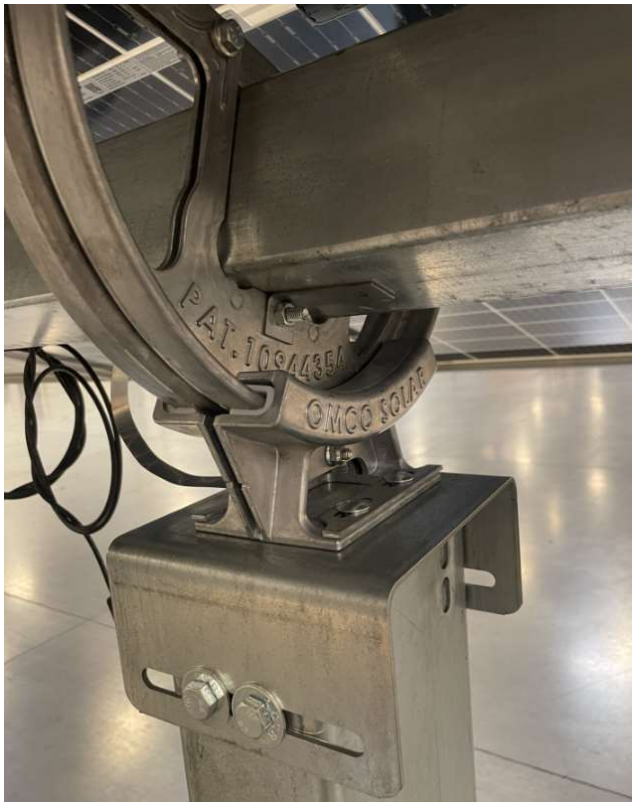
Figure 2: Test Sample Installed Prior to loading
