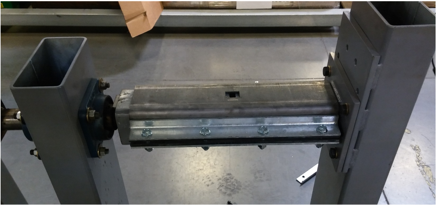
Figure 2: Close-up of Mega Splice Test Sample
