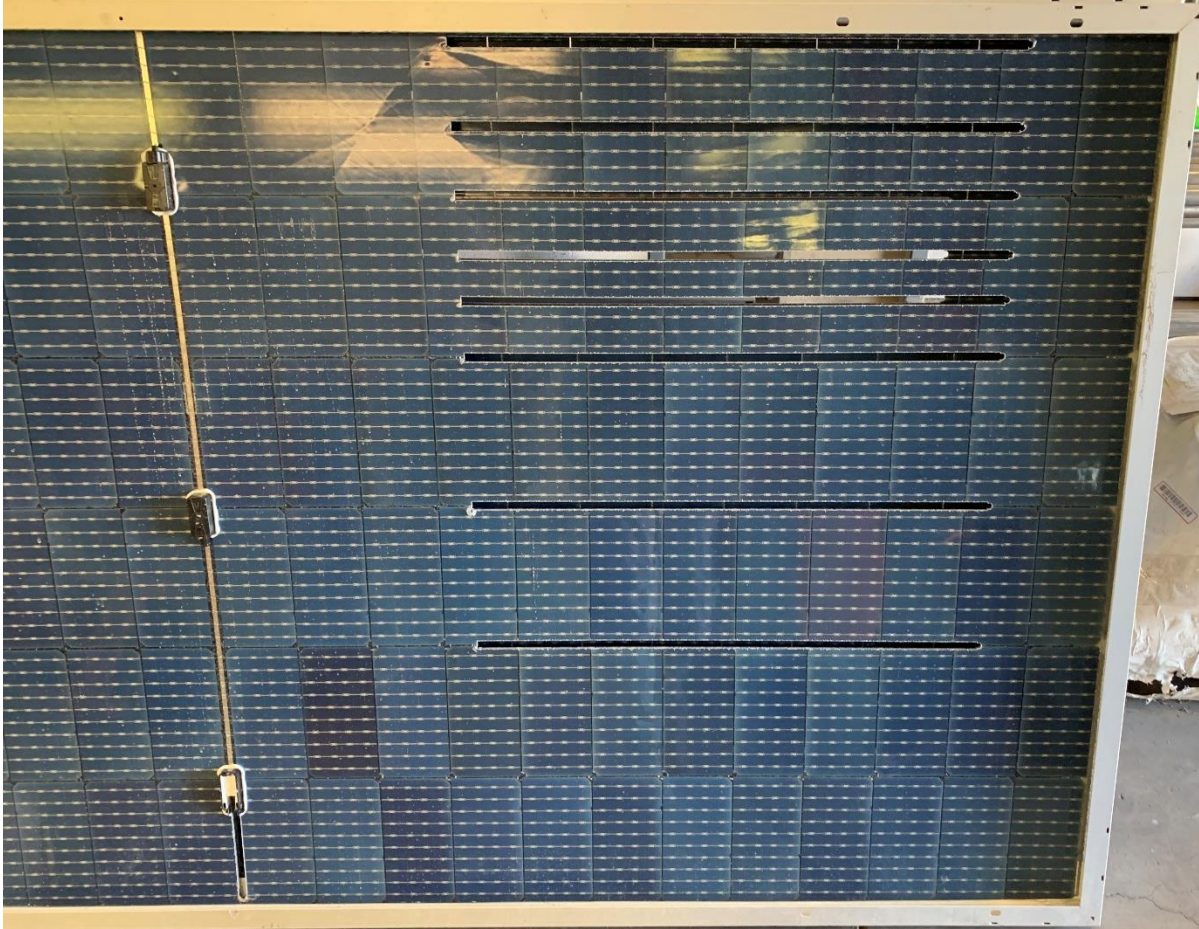
Fig 4: Module post-waterjet cutting process
