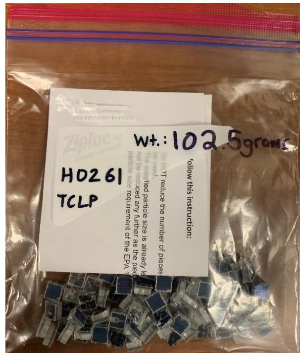
a. TCLP samples prepared for modules HLS0259 (104.5 g) and HLS0261 (102.5 g)
