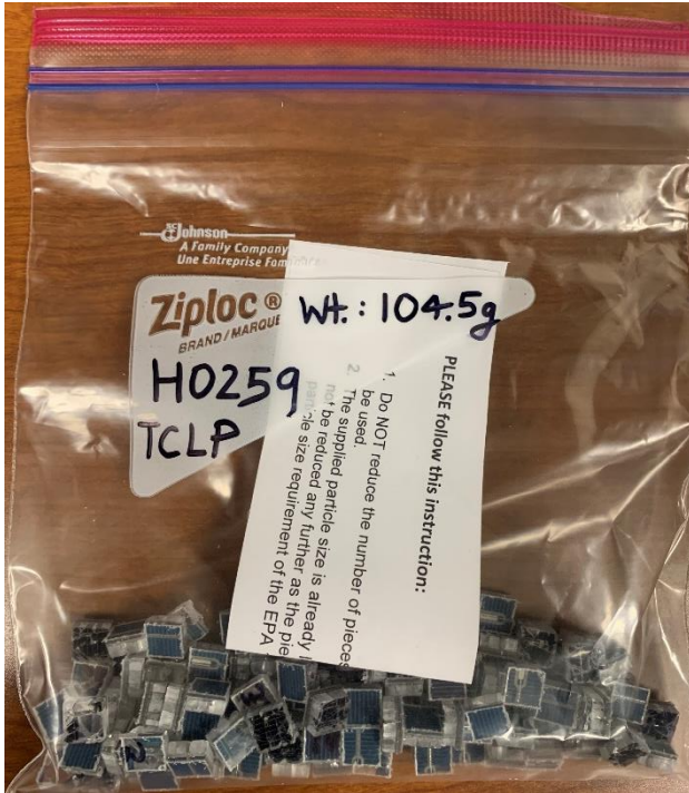
a. TCLP samples prepared for modules HLS0259 (104.5 g) and HLS0261 (102.5 g)
