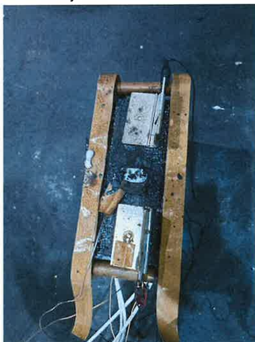
Sample #2: After thermal runaway test
