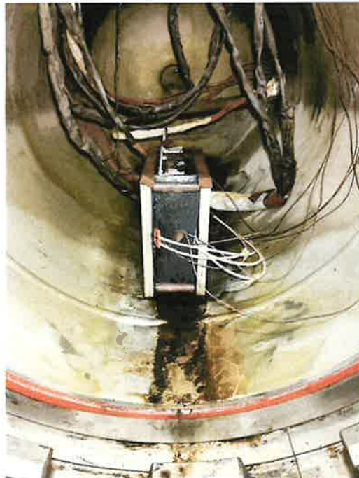
Sample #1: After thermal runaway test
