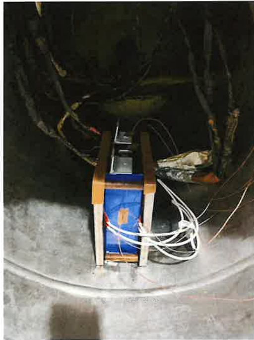
Sample #1: After thermal runaway test
