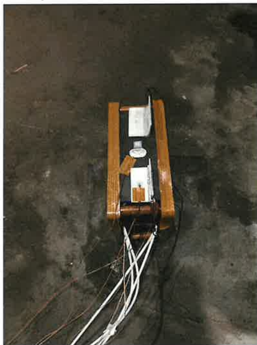
Sample #2: Thermal runaway test setup
