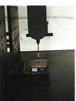
Penetration with heated nail
