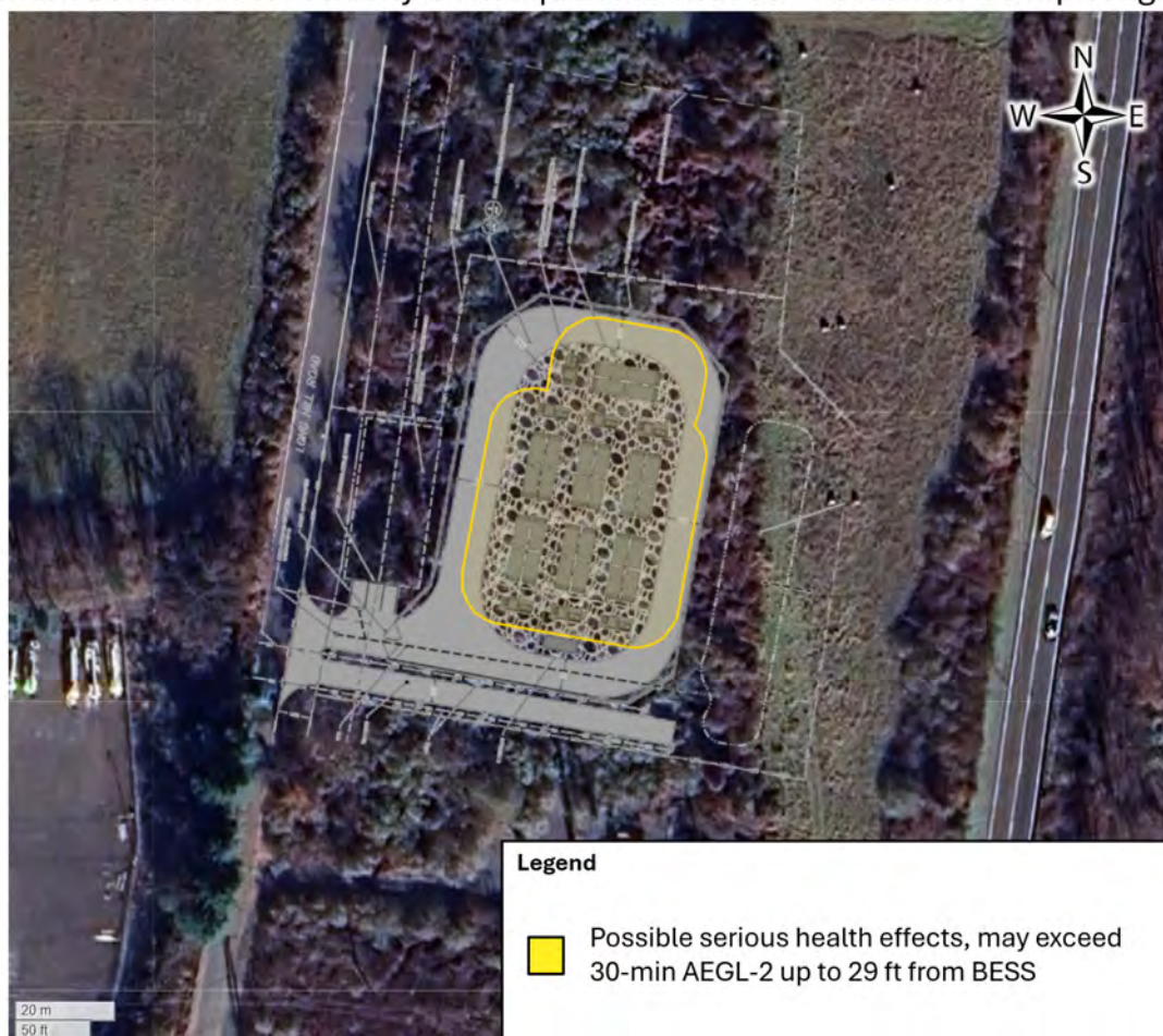
Figure 22: Satellite imagery of the immediate site surroundings with an overlaid area containing possible AEGL-2 levels of toxic gases with steady 8 m/s (18 mph) wind, which is the 99th percentile wind speed for the Long Hill BESS site. No toxicity consequences were present for the modeled scenarios with low wind conditions. Note that these buffers do not account for possible hydrogen fluoride concentrations. This image was produced using Open Street Map and Google Maps.
