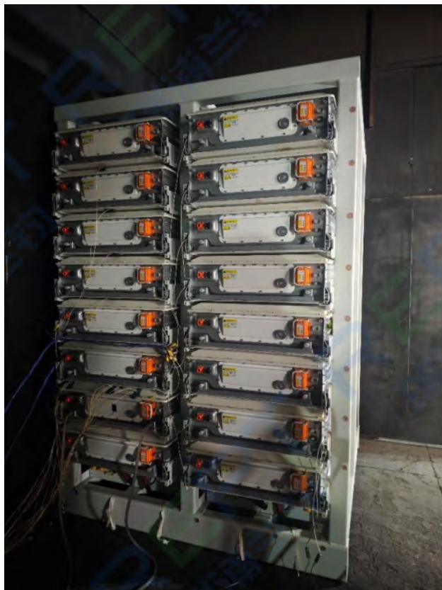
Figure 11: A picture of the unit test setup. This image was taken from the UL 9540A unit-level test report [4].
