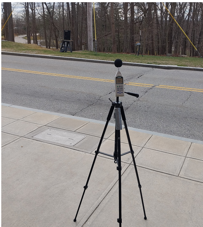
Figure 1. Soundboks Speaker at PM-2 Position and Sound Level Meter at Nathan Hale Hall
