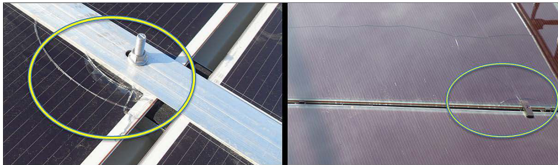
Fig. 4.3.1: Left figure shows glass breakage caused by too tight screws and the right figure a PV module that broke due to poor clamp design.
